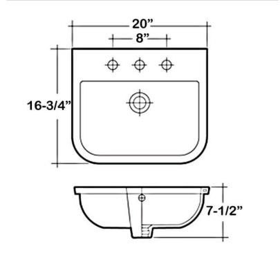
Dimensions of fixture are nominal and may vary within the range of tolerances established by ANSI Standard A112.19.2-2018. Dimensions and specifications subject to change without notice.
